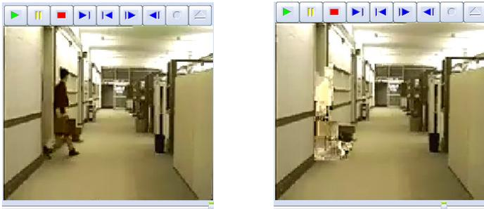
**Fig. 2.** (a) Decoded image with the right key (b) Scrambled image with a wrong key
