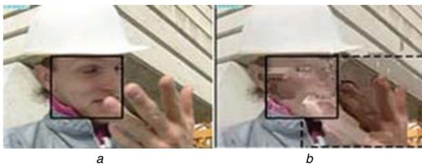
**Fig. 2** 155th frame of Foreman scrambled with drift error
