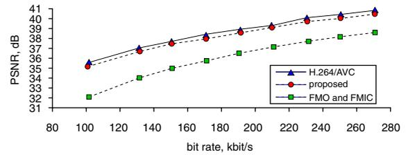
**Fig. 6** Rate distortion performance comparison for Foreman sequence
