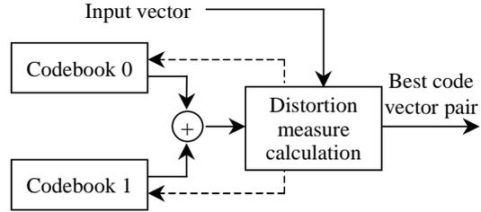
Fig. 3. Conjugate-structure vector quantization scheme
